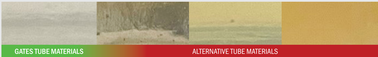
PG25 COOLANT AFTER EXTRACTABLES TESTING WITH VARIOUS DATA CENTER HOSES AT 80°C FOR 600 HOURS
