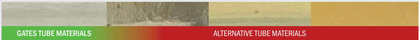
PG25 COOLANT AFTER EXTRACTABLES TESTING WITH VARIOUS DATA CENTER HOSES AT 80°C FOR 600 HOURS
